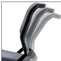
Back-Tilt - As you recline, the torsion-bar back flex mechanism gradually increases resistance over the entire 12° range.
